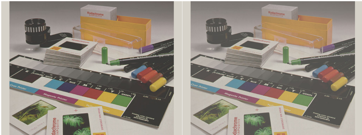
Appearance of an actual newsprint sample in a viewing booth (left) and its typical washed-out proof (right).
