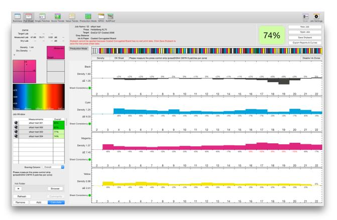
For offset printing processes it is recommended that, once the process inks are an acceptable  $\Delta E$ , the RGB overprints also be checked for Trapping % and  $\Delta E$ . If they are out of tolerance then adjustments to press settings or consumables may be required, which can affect the plate compensation required to achieve the neutral print density curve.
