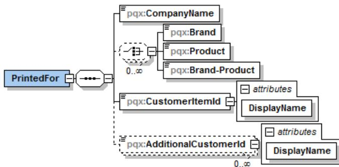
Figure 6.1 PQX “Printed For” Block Structure
