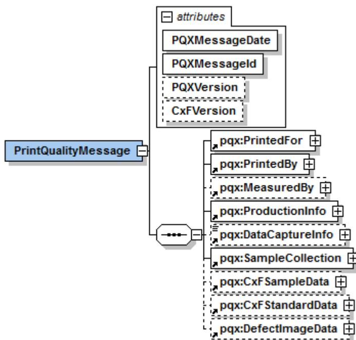
Figure 4.1 High Level PQX Structure
