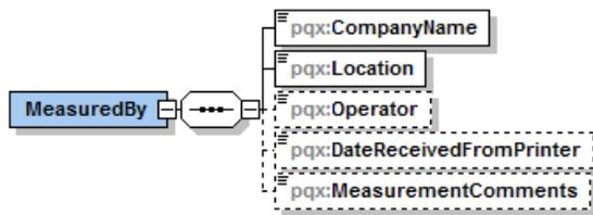
Figure 6.3 PQR “Measured By” Block Structure.
