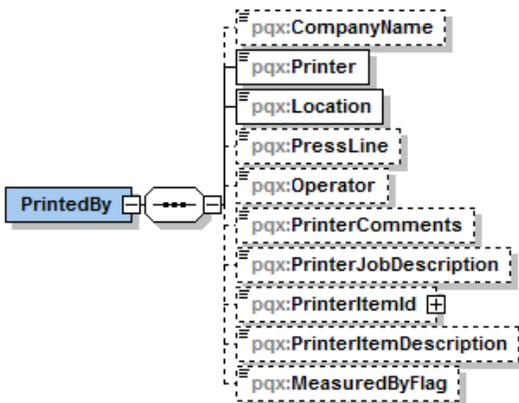
Figure 6.2 PQX “Printed By” Block Structure
