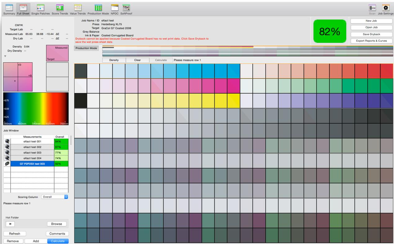
Start with line 1 and measure sequentially. The software automatically selects the next line after each scan. The "active" line to be measured is highlighted with an orange border.
