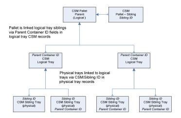
Scan to Pallet operation is supported as long as a physical tray scanned has already been linked to a logical CSM record. At the time of the scan, the link from the logical tray CSM record and the pallet can be established. In fact, only one physical tray associated with a logical tray need be scanned to establish the link for all physical trays. Limitation: If there are multiple physical trays associated with a logical tray, they must go on the same pallet.
